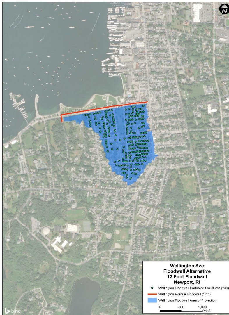
Figure 5-4: Wellington Avenue Structural Alternative Area of Protection
